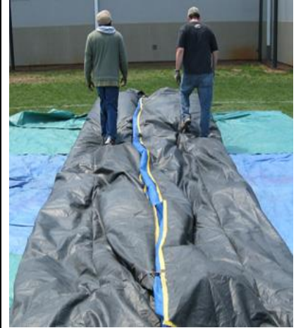
Step 2-6: Fold the Inflatable in 2-3 feet lengthwise & walk out air towards Ports (Blower tubes).
